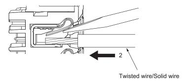
**3** Remove the flat-blade screwdriver from the release hole.
