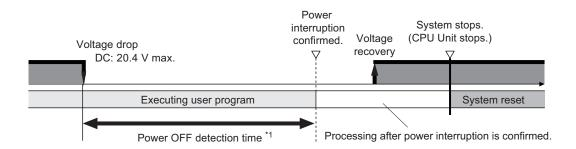
\*1. The power OFF detection time is 2 to 4 ms.
