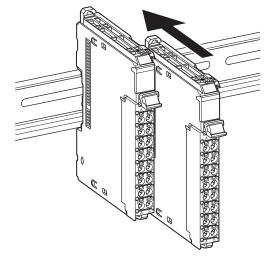
**3** Press the NX Unit with a certain amount of force against the DIN Track until you hear the DIN Track mounting hook lock into place.
