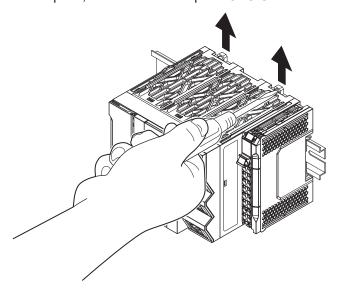
Remove the CPU Unit from the DIN Track.
