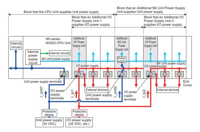
\*1. The minimum value is selected among the rated currents of the multiple I/O power supply units connected to the protective device. If, for example, two rated currents of 10 A and 4 A are used, 4 A will be selected.
