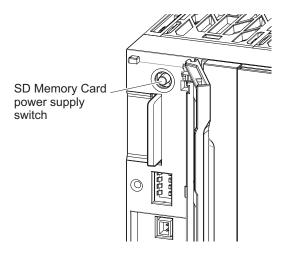
Press the SD Memory Card after you confirm that the SD BUSY indicator (lit while SD Memory Card access is in progress) and SD PWR indicator (lit while SD Memory Card power is supplied) are no longer lit.
