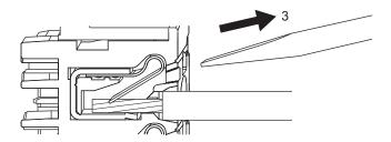
After you make a connection, lightly pull the twisted wire or the solid wire to make sure that the wire is securely connected to the terminal block.
