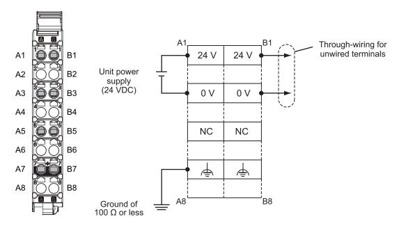
Connect the DC power supply to the Unit power supply terminals.
