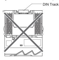
Mounting with the DIN Track Installed Vertically
