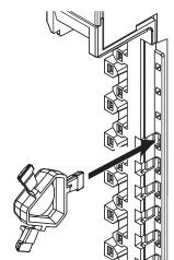
**2** Rotate the runner to break off the Coding Pin.
