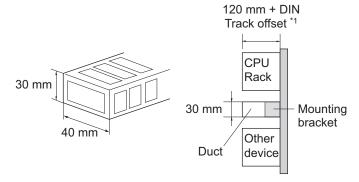
\*1. It varies depending on the DIN Track to be used. Refer to *Installation Dimensions* on page 5-33 under 5-3-14 Assembled Appearance and Dimensions on page 5-33 for details. It corresponds to the dimension (B).
