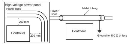
Example: Separating Controller from Power Lines
