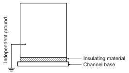
Example: Insulating and Grounding an Enclosure
