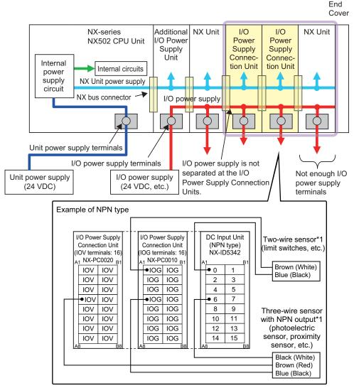
\*1. Wire colors have been changed according to revisions in the JIS standards for photoelectric and proximity sensors. The colors in parentheses are the wire colors prior to the revisions.
