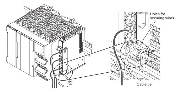
**3** Bundle wires with a cable tie and secure them to the screwless clamping terminal block.
