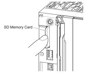
The SD Memory Card will be ejected from the compartment.
