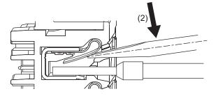
3. Leave the flat-blade screwdriver tilted and pull out the ferrule.
