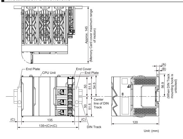
W: Width of CPU Unit (including the End Cover)
