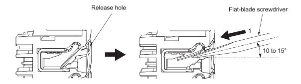
**2** Leave the flat-blade screwdriver pressed into the release hole and insert the twisted wire or the solid wire into the terminal hole.
