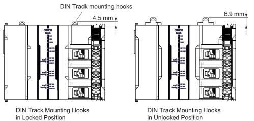
If the DIN Track mounting hooks are pulled up, they are in the unlocked position. If the DIN Track mounting hooks are pressed down, they are in the locked position.
