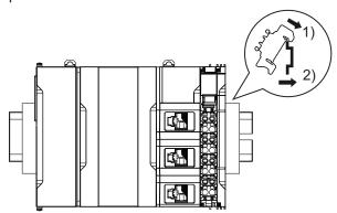
To remove an End Plate 1) insert the tip of a flat-blade screwdriver into groove "a" and 2) use "b" as a fulcrum and lift the end of the screwdriver, as shown in the following diagram.
