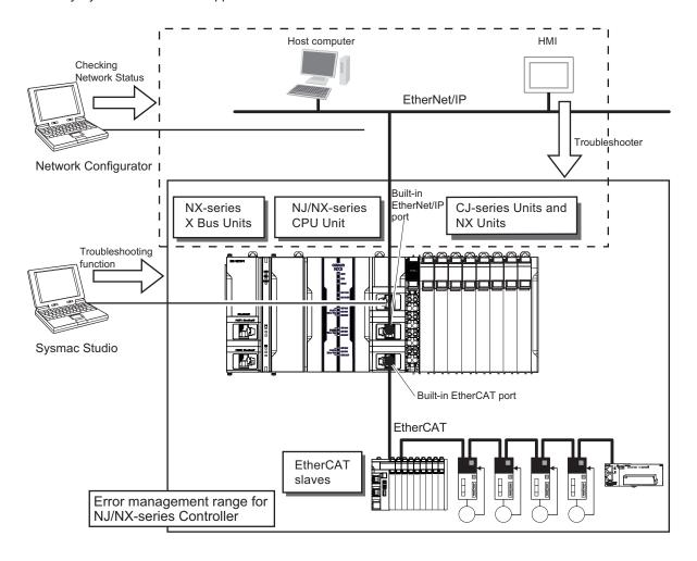
You can use the troubleshooting functions of the Sysmac Studio or the Troubleshooter on an HMI to quickly check for errors that have occurred and find corrections for them.
