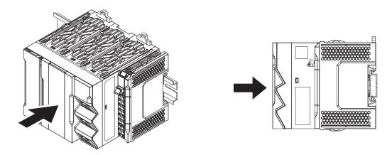
4 Press the DIN Track mounting hooks down to the locked position.
