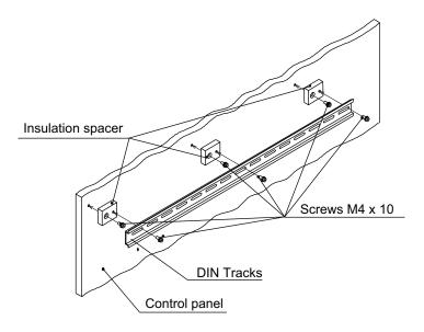
DIN Track Insulation Spacers NX-AUX01 (OMRON Corporation)
