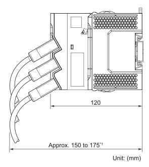
\*1. This is the dimension from the back of the Unit to the communications cables.
