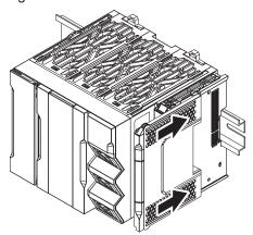
**2** Press the End Cover firmly against the DIN Track until you hear it lock into place on the DIN Track.
