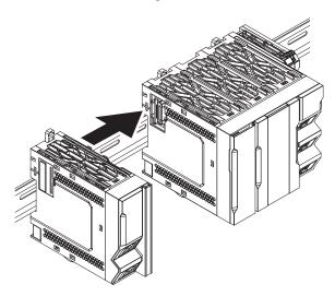
**3** Slide and lock the DIN Track mounting hooks and the upper and lower sliders of the Unit until they click.
