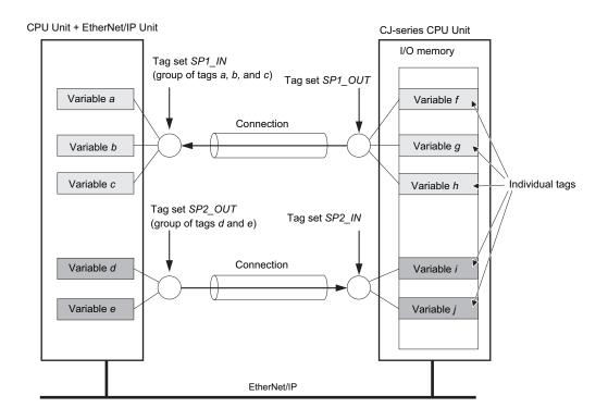
**Note** To enable a connection, each tag set must include only one of ether input tags or output tags. (Both input and output tags cannot be included in one tag set.)
