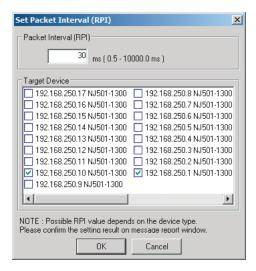
The usage rate of allowable tag data link bandwidth for each of the two devices, 192.168.250.1 and 192.168.250.10, increases to 87.00% as shown in the Usage of Capacity column, and this indicates that the shorter RPI is set for the connections of these devices.
