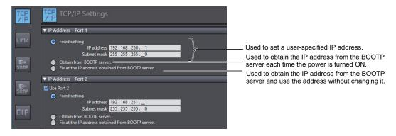
The IP addresses must be set separately for EtherNet/IP ports 1 and 2.
