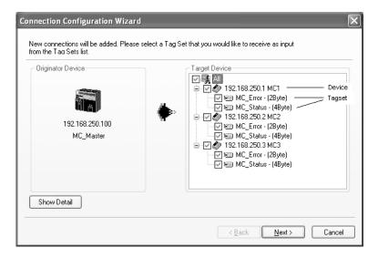
4 A list of tag sets is displayed on the right side of the Wizard with target devices that support receiving input data.
