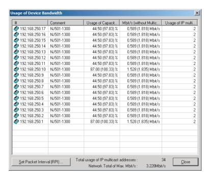
In this case, if the Ethernet switch has no multicast filter, the Usage of Capacity value would be 100.33% and communications errors might occur due to traffic overload at the EtherNet/IP port.
