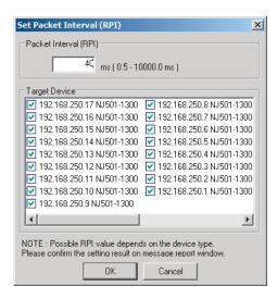
If you set the same packet interval (RPI) for all the connections, the table shows that the usage rate of allowable tag data link bandwidth is 74.50% for all the device as shown in the Usage of Capacity column, and this indicates that the shortest packet interval is 40 ms.
