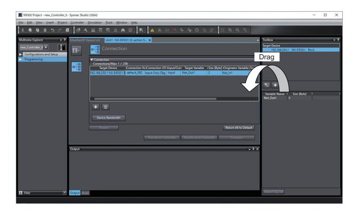
Specify Originator Variable and its Size [Byte] for the tag set Net\_Out1 added in step 5. Here, specify Net\_In1 for Originator Variable and 2 for its Size [Byte]. Change the other settings as required.
