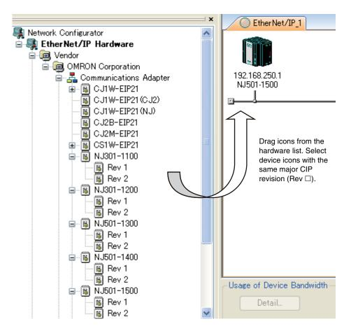
The device names and major CIP revisions (Rev  $\square$ ) are displayed in the hardware list. For the NJ/NX-series Controllers, device names of Units and major CIP revisions are as shown in the following table.
