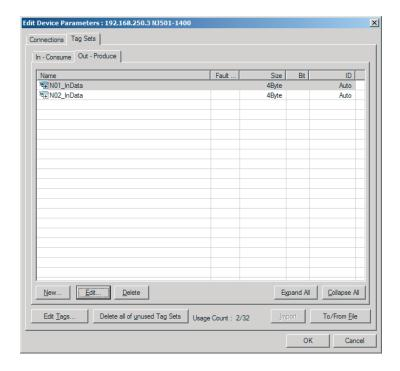
To place more than one input variable (input tag) imported from the Sysmac Studio into one tag set, you must delete the input tags that were registered.
