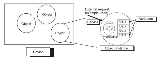
In the CIP Common Specification, Object, Class, Instance, Attribute, and Service are defined as follows: (Source: CIP Common Specification)
