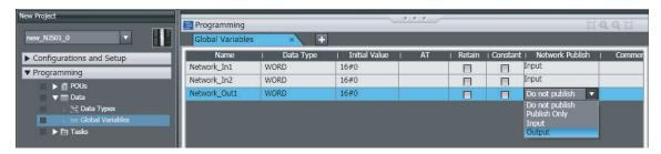
Select Export Global Variables - Network Configurator... from the Tools Menu. Any global variables with Input or Output set for the Network Publish attribute are imported from the csv file through the import procedure described below (Importing to the Network Configurator).
