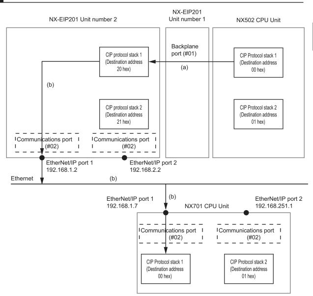
The network type numbers and the destination addresses for routes (a) and (b) in the above figure are as shown in the table below.
