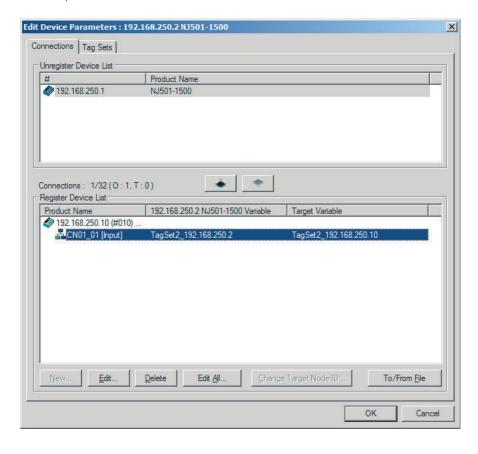
4) The Edit Connection Dialog Box for the device is displayed. Input a new packet interval (RPI) value, and click the **OK** Button.
