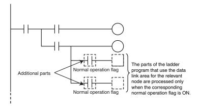
• The following shows an example where data processing is performed only when data links are operating normally with MC and MCR instructions, or with JMP instructions.
