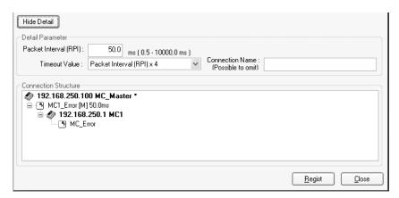
The specified values for detailed parameters will be displayed. Change the values as required. Connection names are automatically created using the following rule. default N (where N is a 3-digit number (001, 002, etc.) starting from 1)
