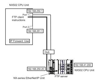
When the CPU Unit executes the FTP client instruction specifying the NX5 CPU Unit with IP address 192.168.41.200, an IP packet is transferred to the NX5 CPU Unit, which is the FTP server, via the EtherNet/IP port 1 on the NX-series EtherNet/IP Unit in the same network segment.
