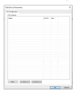
**3** Click the **New** Button from the **I/O Configuration** Tab Page. The **Edit I/O Instance** Dialog Box is displayed.
