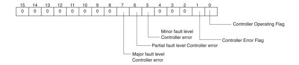
**Note** Of the flags in bits 5 to 7 that indicate the current error level, only the flag for the highest error level changes to TRUE.
