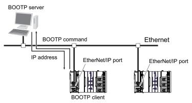
The EtherNet/IP port IP address is obtained from the BOOTP server when the power is turned ON.
