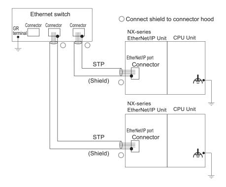
Connecting the shields only at the Ethernet switch sideConnect the shields to the connector hoods only at the Ethernet switch side.
