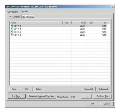
2 If an input tag is already registered in an input tag set, and you want to change its registration to a different input tag set, it is necessary to delete the tag from the tag set in which it was originally registered.
