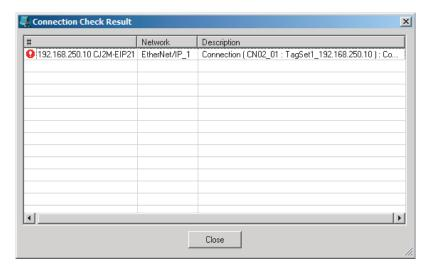
If an inconsistency is found, open the originator's **Edit Device Parameter** Dialog Box and click the **Connection** Tab. The inconsistent connection in the **Register Device List** is displayed
