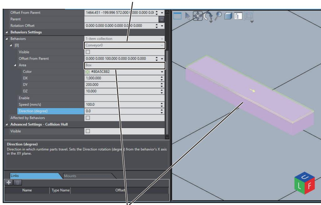
Area where a part should be operated when it comes in contact with the 3D shape data
