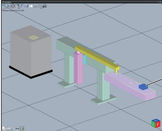
A box simulating the conveyor carries the part.
