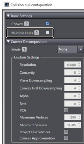
However, when a 3D shape data is made up of a single or a few objects as shown in the following figure, selecting the **Multiple Hulls** check box is not very effective. To increase the accuracy of collision detection, change the accuracy of collision hulls in the Collision hull configuration dialog box.
