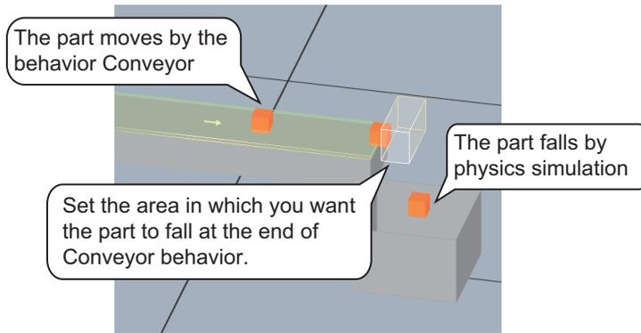
**5** In 3D shape data that the part will come in contact with after the physics simulation, set the collision detection filter to allow the part to continue its motion. If you do not set this, the part dropped in the physics simulation will pass through even when it collides with the 3D shape data.
