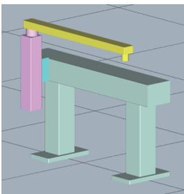
To import CAD data for movable part that consists of a base, an X-axis slider, a Z-axis slider, and an arm with a rotary axis as the mechanical component *X-Y table (XY Theta)*, create a CAD data file for each of the base, X-axis slider, Z-axis slider, and arm with a rotation axis. (In this example, Z axis is applied to the Y axis of the X-Y table (XY Theta).)
