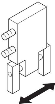
For the Robot tool (Parallel switching 2-finger type chuck/double solenoid type) model, set the following parameters.
