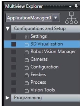
In **3D Visualization** under **Configurations and Setup**, manage the 3D shape data for virtual equipment models, settings for operating the mechanical components and Virtual Part Detection Sensor, and scripts that define the operations of the parts that you want to use for 3D simulations.
