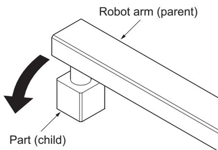
To set a parent-child relationship, select the parent 3D shape data on the setup tab page for the child 3D shape data.
