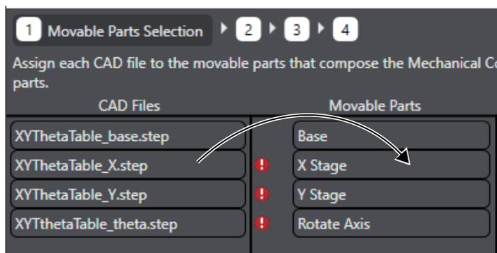
The CAD files are assigned and displayed under the movable parts.
