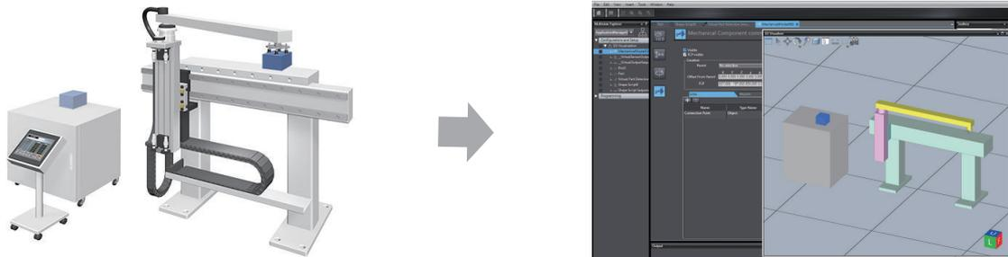
A virtual equipment model consists of a *mechanical component*<sup>\*1</sup> that represents a movable part of the equipment, a *part* that represents the target to be carried, and a *Virtual Part Detection Sensor* that detects the part.
