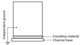
Example: Insulating and Grounding an Enclosure
