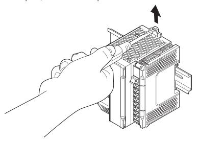
2 Remove the CPU Unit from the DIN Track.
