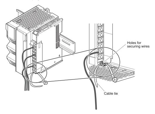
**3** Bundle wires with a cable tie and secure them to the screwless clamping terminal block.
