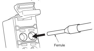
After you make a connection, make sure that the ferrule is securely connected to the terminal block.
