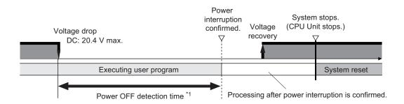
\*1. The power OFF detection time is 2 to 8 ms.
