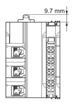
DIN Track Mounting Hooks in Unlocked Position
