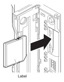
**3** Push the SD Memory Card securely into the compartment.
