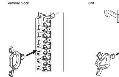
**2** Rotate the runner to break off the Coding Pin.
