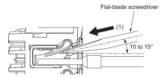
2. Leave the flat-blade screwdriver pressed into the release hole and tilt the flat-blade screwdriver approximately 5° to the direction of the ferrule.
