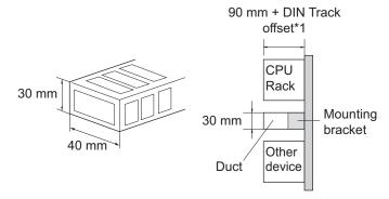
\*1. It varies depending on the DIN Track to be used. Refer to *Installation Dimensions* on page 5-31 under 5-3-12 Assembled Appearance and Dimensions on page 5-31 for details. It corresponds to the dimension (B).
