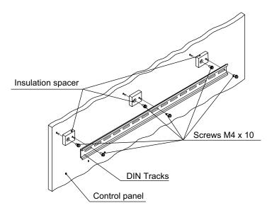
DIN Track Insulation Spacers NX-AUX01 (OMRON Corporation)
