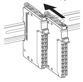
**3** Press the NX Unit with a certain amount of force against the DIN Track until you hear the DIN Track mounting hook lock into place.
