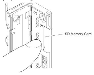
The SD Memory Card will be ejected from the compartment.
