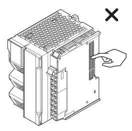
Do not write anything with ink within the restricted region of the CPU Unit that is shown in the following figure. Also do not get this area dirty. When the Unit is installed or removed, ink or dirt may adhere to the pins in the NX bus connector, which may result in malfunctions in the Unit.
