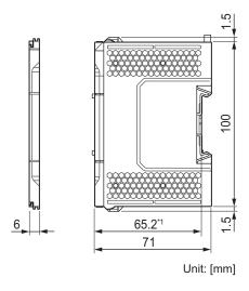
\*1. The dimension from the attachment surface of the DIN Track to the front surface of the end cover.
