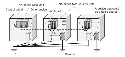
b. Installation method by connecting devices and noise sources to a common earth electrode This is an earthing method to connect the device that is connected with a communications cable, other devices, and a device that could be a noise source, to a common earth electrode. This earthing method is not recommended, because the device that is a potential noise source may interfere electromagnetically with other devices.
