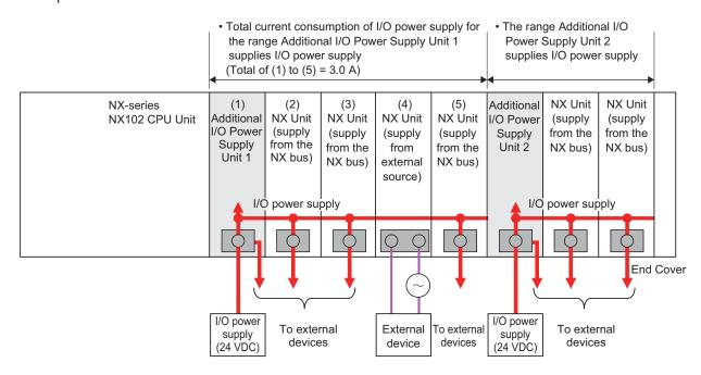
I/O power supply current consumption of each Unit
