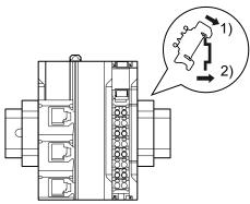
To remove an End Plate 1) insert the tip of a flat-blade screwdriver into groove "a" and 2) use "b" as a fulcrum and lift the end of the screwdriver, as shown in the following diagram.
