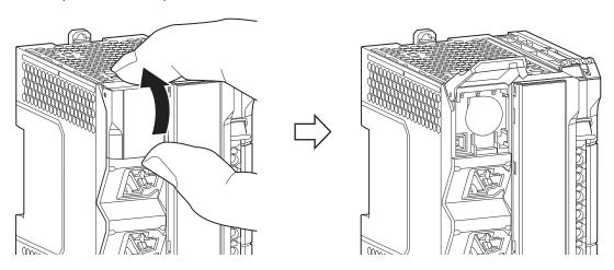
3 Connect the connector of the battery to the battery connector and insert the battery in the battery slot.
