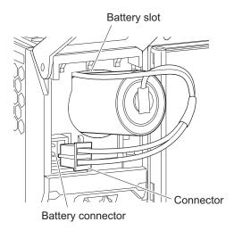
**4** Press in the battery harness by twisting and attach the battery cover.
