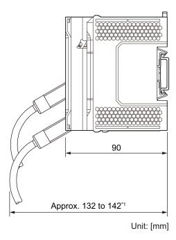
\*1. This is the dimension from the back of the Unit to the communications cables. Approx. 132 mm: When MPS588-C connector is used
