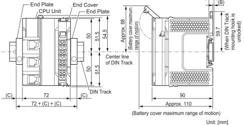
W: Width of CPU Unit (including the End Cover)
