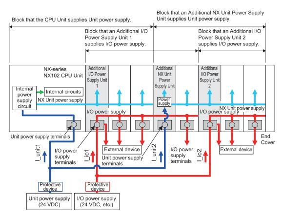
\*1. The minimum value is selected among the rated currents of the multiple I/O power supply units connected to the protective device. If, for example, two rated currents of 10 A and 4 A are used, 4 A will be selected.
