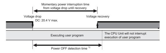
\*1. The power OFF detection time is 2 to 8 ms.
