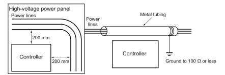
**Example: Separating Controller from Power Lines**
