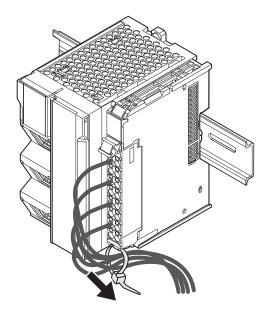
In such a case, secure wires within the range of 30 mm from the screwless clamping terminal block. Also, leave spaces below the CPU Rack to ensure ventilation, as shown in the following figure.
