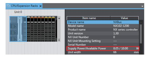
If the power to supply exceeds the NX Unit power supply capacity of the Unit that is selected to supply the NX Unit power, a yellow warning icon is displayed by the first NX Unit for which there is not sufficient capacity and also by all the remaining NX Units.
