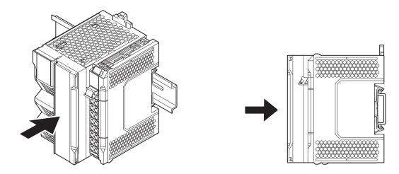
4 Press the DIN Track mounting hooks down to the locked position.
