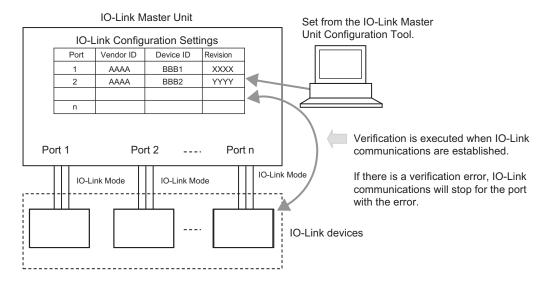
You can verify the vendor ID, device ID, serial number, and IO-Link revision of the connected IO-Link device for each port using either of the following two patterns.
