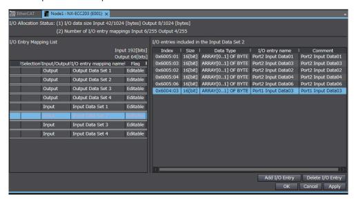
To save the I/O data size for unused ports, delete the I/O entries for the unused ports from the I/O entry mapping list.
