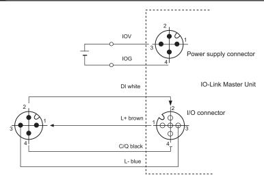
**Note** Even if you connect to IO-Link devices without digital inputs for pin 2, connect pin 2 as shown in the above figure. This is because connectors on the IO-Link devices and the cable with connectors on both ends connect pin 2. However, because no data enters pin 2 of the IO-Link Master Unit, digital IO-Link input data is always OFF.
