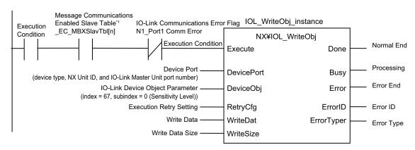
\*1. Use this when you connect the IO-Link Master Unit to a Communications Coupler Unit. This is not necessary when you connect the IO-Link Master Unit to a CPU Unit.
