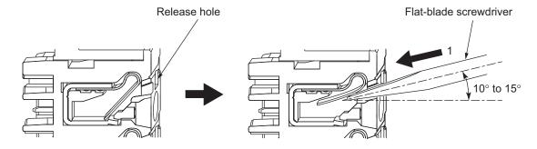
**2** Leave the flat-blade screwdriver pressed into the release hole and insert the twisted wire or the solid wire into the terminal hole.
