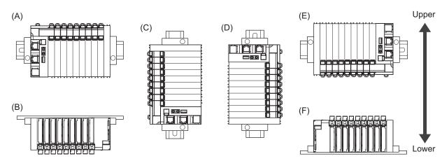
However, there are restrictions on the installation orientation and restrictions to the specifications that can result from the Communications Coupler Units and NX Units that are used.
