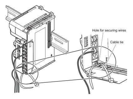
**3** Bundle the wires with a cable tie and secure them to the screwless clamping terminal block.
