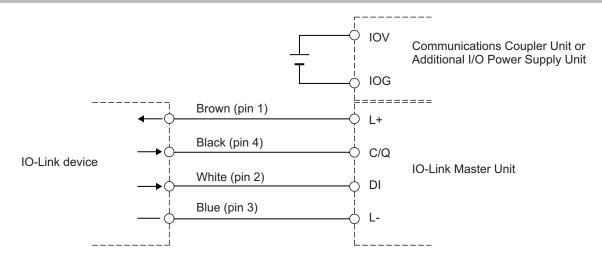
Note 1. If you do not use a signal connection for digital inputs for pin 2, a DI (white) connection is not required.
