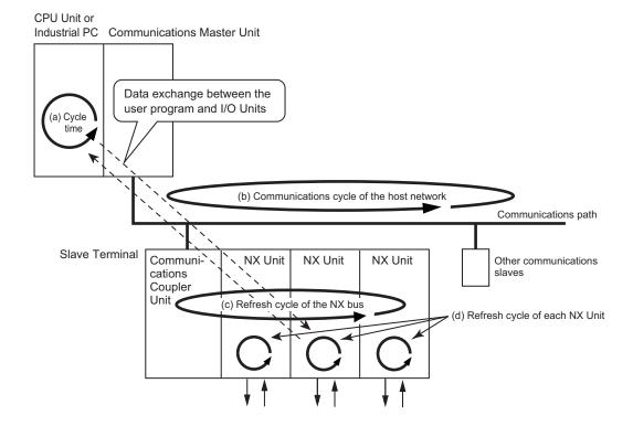
The cycle time of the CPU Unit or Industrial PC and communications cycle of the host network and the I/O refresh cycle of the NX bus are determined by the CPU Unit or Industrial PC types and the communications types.
