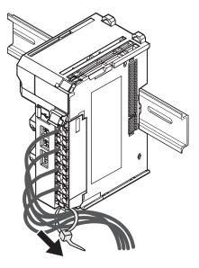
Secure wires within the range of 30 mm from the screwless clamping terminal block.
