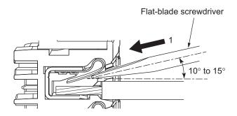
2 Insert the flat-blade screwdriver into the release hole and remove the wire from the terminal hole.
