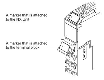
The marker attachment locations vary depending on the type of the external connection terminals on the NX Units.
