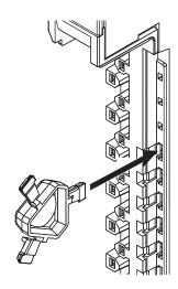
**2** Rotate the runner to break off the Coding Pin.
