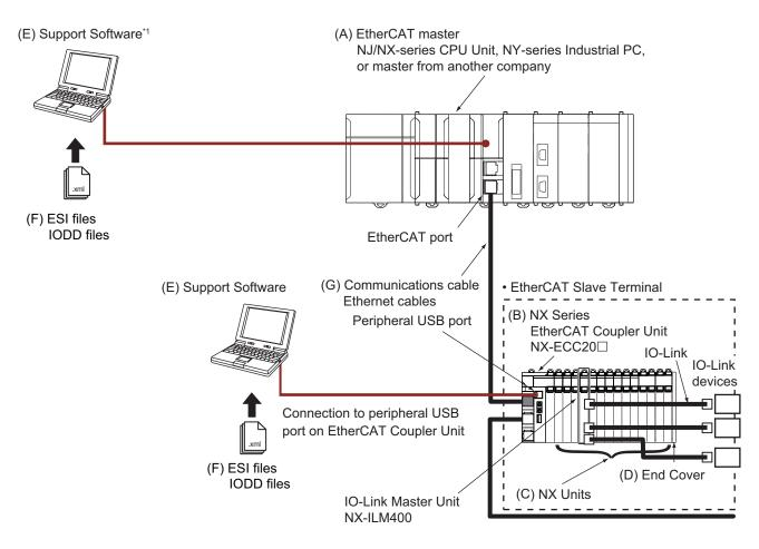
\*1. The connection method for the Support Software depends on the model of the CPU Unit or Industrial PC.
