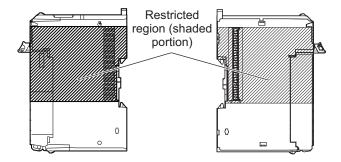
• For the installation orientations in the following figure, support the cables, e.g., with a duct, so that the End Plate on the bottom is not subjected to the weight of the cables. The weight of the cables may cause the bottom End Plate to slide downward so that the Slave Terminal is no longer secured to the DIN Track, which may result in malfunctions.
