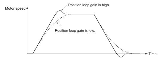
• If the speed loop gain and position loop gain are optimally set, the motor operation for the command delays 2/Kp at acceleration and delays 3/Kp at deceleration.
