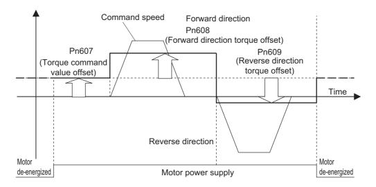
The Torque Command Value Offset (Pn607) reduces the variations of positioning operations due to the movement directions when a certain amount of unbalanced load torque is always applied to the motor at the vertical axis by setting the torque command.
