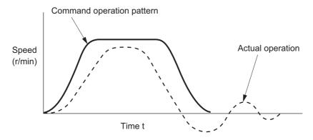
• If the speed loop gain is high, vibrations are more likely to occur. Vibration or resonance may not disappear.
