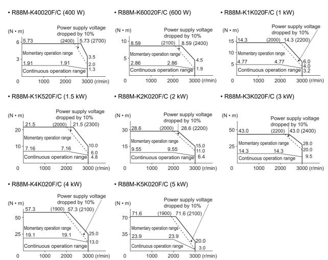
Note: The continuous operation range is the range in which continuous operation is possible. Continuous operation at the maximum speed is also possible. However, doing so will reduce the output torque.
