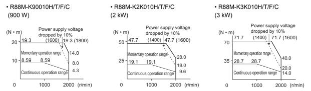
Note:The continuous operation range is the range in which continuous operation is possible. Continuous operation at the maximum speed is also possible. However, doing so will reduce the output torque.
