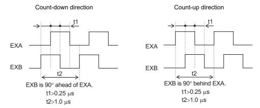
\*3. For the external encoder connection direction, set the rotation direction so that count-up occurs when the motor shaft is rotating in the CCW direction, and count-down occurs when the motor shaft is rotating in the CW direction. If the connection direction cannot be selected due to installation conditions, etc., the count direction can be reversed using External Feedback Pulse Direction Switching (Pn326).
