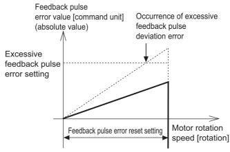
• Ensure that an appropriate value is set to the Internal/External Feedback Pulse Error Counter Reset (Pn329), before you use the feedback pulse error counter reset. When the set value is extremely small, the protective function may not work to prevent any erroneous operation due to improper connection of the external encoder.
