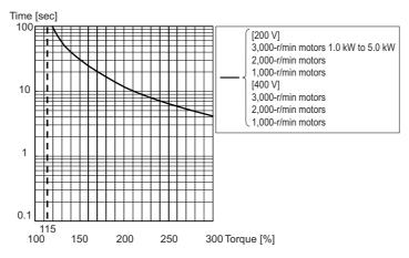
When the torque command = 0, and a constant torque command is continuously applied after 3 or more times the overload time constant has elapsed, the overload time t [s] is:  $t [s] = -\text{Overload time constant} [s] \times \log_e (1 - \text{Overload level [\%]} / \text{Torque command [\%]})^2$  (The overload time constant [s] depends on the motor. The standard overload level is 115%.)
