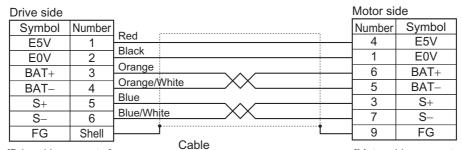
[Drive side connector] Connector model
