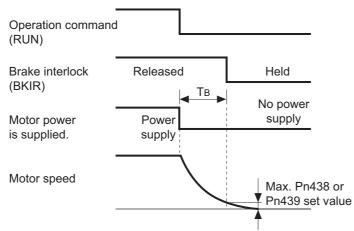
The Time ta in above drawing is either the Brake timing during operation (i.e., the set value  $\times$  1 ms) or the time taken until it goes below the value set on the Brake Release Speed Setting (Pn439), whichever is shorter. For details, refer to "6-5 Brake Interlock (P.6-14)".
