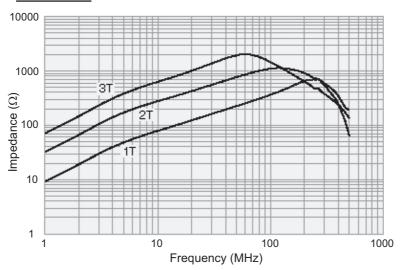
Refer to the following sections for the dimensions and impedance characteristics of the ZCAT3035-1330: "External Dimensions" (P.4-32) and "Impedance Characteristics" (P.4-38).
