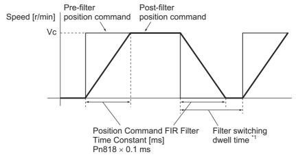
\*1. Change the setting on Pn818 only after you stop the command pulse and the filter switching dwell time elapses. The dwell time is calculated by the following formulas depending on the value set on Pn818.
