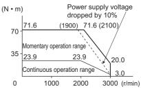
Note: The continuous operation range is the range in which continuous operation is possible. Continuous operation at the maximum speed is also possible. However, doing so will reduce the output torque.
