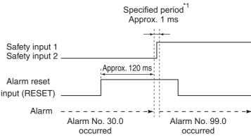
\*1. Alarm No. 99.0 will occur if at least one of the input photocouplers for safety inputs 1 and 2 is turned from OFF to ON.
