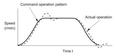
• If the position loop gain is low, positioning completion speed becomes slow.
