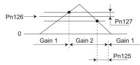
• The settings for the Gain Switching Level in Torque Control (Pn126) and the Gain Switching Hysteresis in Torque Control (Pn127) are enabled as absolute values (positive/negative).
