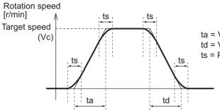
ta = Vc / Maximum motor rotation speed  $\times$  Pn312  $\times$  1 ms td = Vc / Maximum motor rotation speed  $\times$  Pn313  $\times$  1 ms ts = Pn314  $\times$  1 ms
