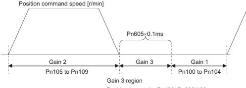
Position loop gain=Pn100×Pn606/100 Speed loop gain=Pn101×Pn606/100
