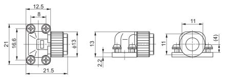
Angle clamp model JN6FR07SM1 (Japan Aviation Electronics) Connector pin model LY10-C1-A1-10000 (Japan Aviation Electronics)
