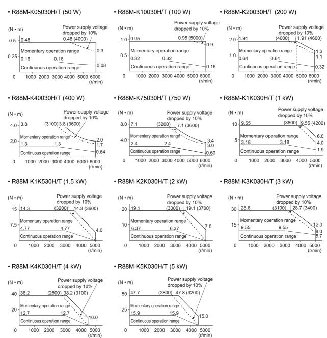
Note:The continuous operation range is the range in which continuous operation is possible. Continuous operation at the maximum speed is also possible. However, doing so will reduce the output torque.
