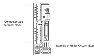
1. Remove the terminal block from the Servo Drive before wiring.
