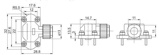
Angle plug model JN8FT04SJ1 (Japan Aviation Electronics)
