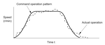
• If the speed loop integral time constant is high, the response is delayed. The servo rigidity becomes weak.
