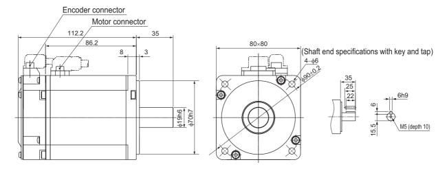
Note. The standard models have a straight shaft. Models with a key and tap are indicated with S2 at the end of the model number.
