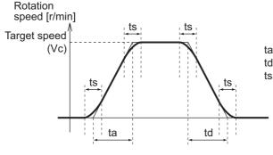
ta = Vc / Maximum motor rotation speed  $\times$  Pn312  $\times$  1 ms td = Vc / Maximum motor rotation speed  $\times$  Pn313  $\times$  1 ms ts = Pn314  $\times$  1 ms
