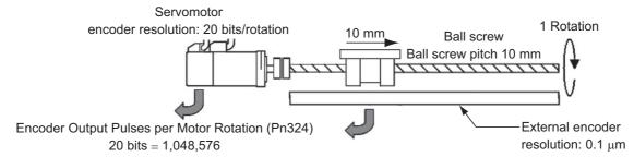
External encoder Output Pulse Per Motor Rotation (Pn325)  $10 \text{ [mm]} / 0.1 \text{ [}\mu\text{m/pulse]} = 100,000 \text{ [pulse]}$
