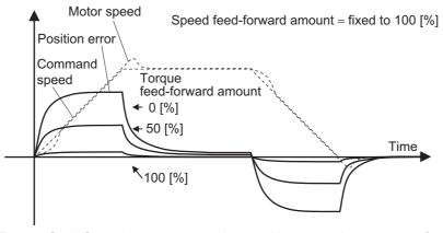
Torque feed forward can reduce the position error in a range of acceleration/deceleration specified.
