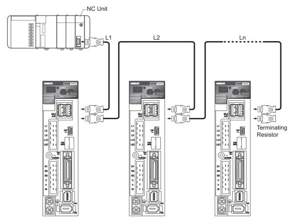
Note 1.The cable between the two nodes (L1, L2  $\dots$  or Ln) must be 0.5 m or longer. Note 2.The total length of the cable (L1 + L2 +  $\dots$  Ln) must be equal to or shorter than 50 m.
