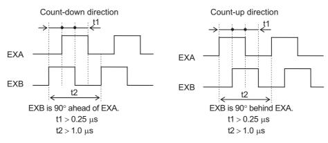
\*3 For the external encoder connection direction, set the direction so that count-up occurs when the motor shaft is rotating in the CCW direction, and count-down occurs when the motor shaft is rotating in the CW direction If the connection direction cannot be selected due to installation conditions, etc., the count direction can be reversed using External Feedback Pulse Direction Switching (Pn326).
