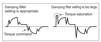
When the Damping Frequency 1 (Pn214) is set, reduce the setting if torque saturation occurs or increase the setting to increase operation speed. Normally 0 is set.
