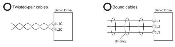
• Separate power supply lines and signal lines when wiring.
