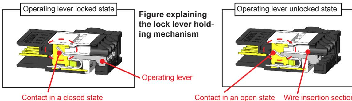
Wires are not held in place as the operating lever is in an unlocked state.
