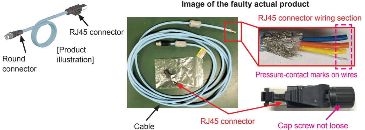
The cable was pressure-contacted to the connector (i.e. connected state) and was disconnected from this state.
