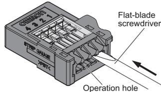
(2) Insert the wire fully to the back of the wire insertion hole. Make sure that the cable sheath is inserted into the hole, and that the end of the wire has passed through the contact section.
