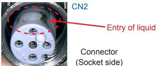
\* It is assumed that a short circuit was caused by liquid entering from the connector fitting which resulted in the body melting.
