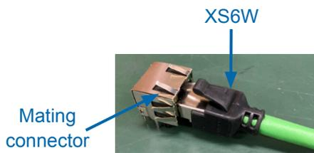
Measurement after fitting the mating connector into an XS6W connector
