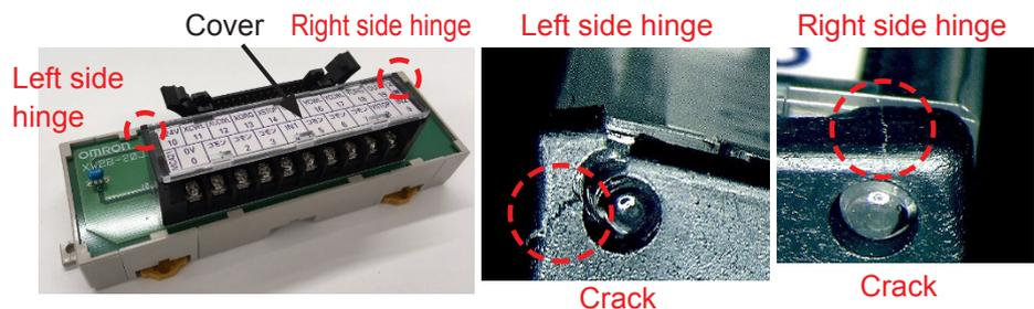
\* In the assembly process of target product, the hinge is not subjected to excessive loads.
