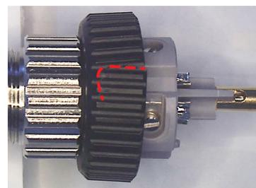
\* Crack occurred along section marked by a red dotted line.
