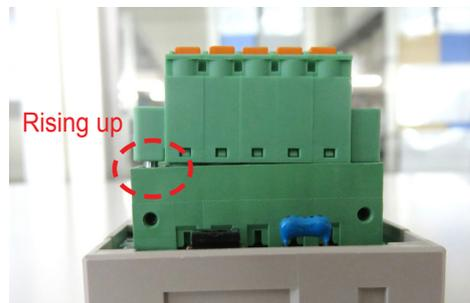
The connector fixing screw on one side rises up as it is not fully tightened.
