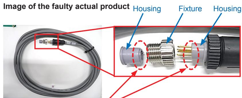
Joint locations (ultrasonic welded sections) of molded parts are damaged and separate.
