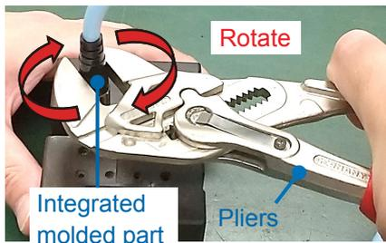
Tighten **the fixture** by hand or using a special tool (at the specified torque). **This way, the housing will not break.**
