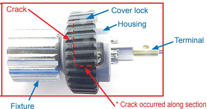
\* Crack occurred along section marked by a red dotted line.
