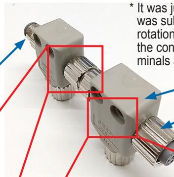
\* It was judged that the connector fitting was subjected to excessive external rotational force that caused damage to the connector and breakage of the terminals and resulted in continuity failure.
