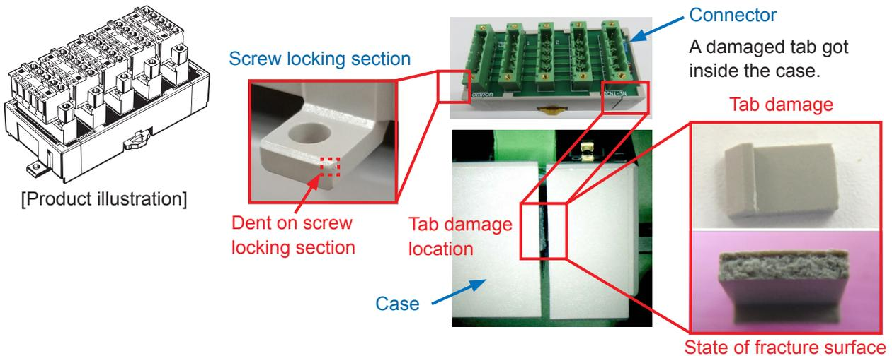
\* The condition of the target product can be detected by visual inspection.
