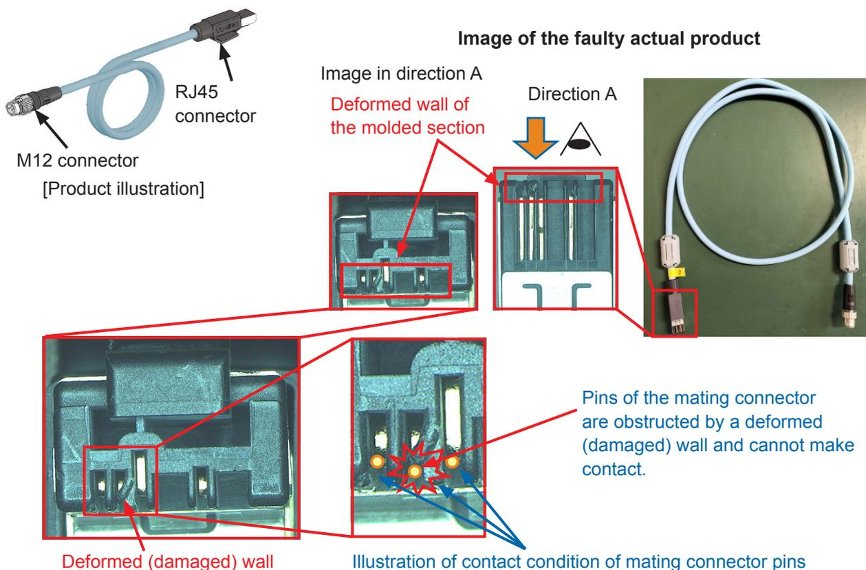
\* All target products are inspected for continuity and withstand voltage, and any abnormality can be detected.
