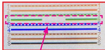
Transmission characteristics are not satisfied due to lack of conduction at deformed location
