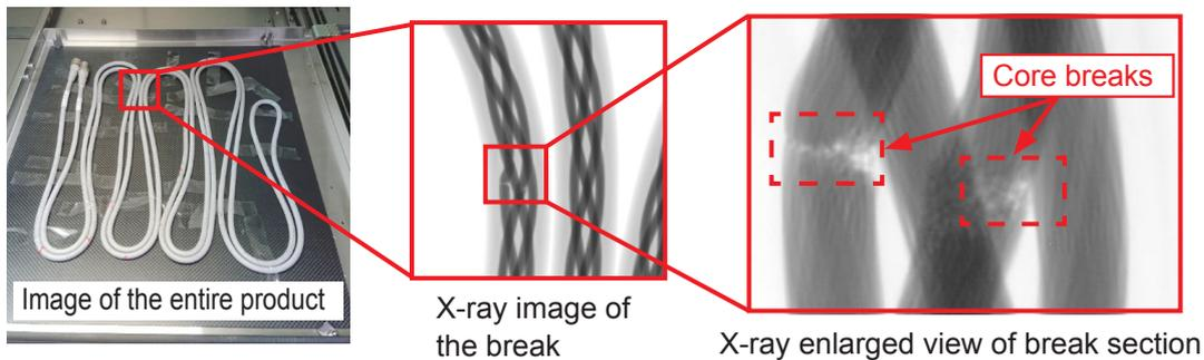
\* All target products are inspected for continuity and withstand voltage, and any abnormality can be detected.
