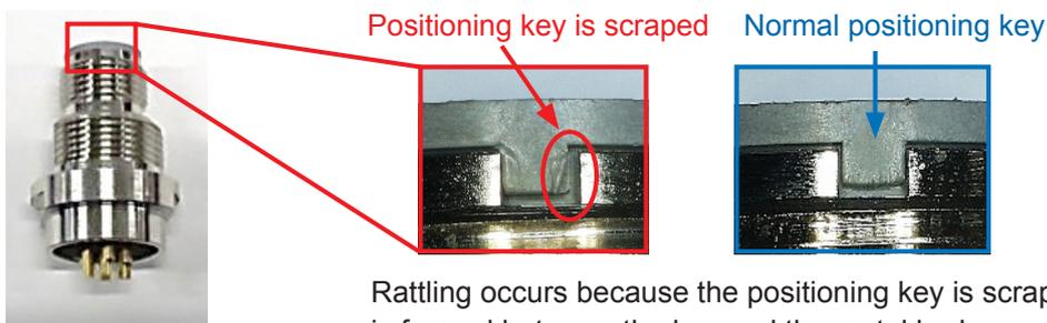
Rattling occurs because the positioning key is scraped and a clearance is formed between the key and the metal body.
