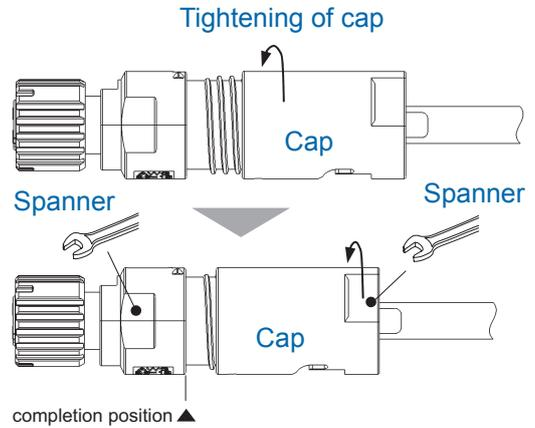
(\*1) If tightened with a tool that has a large width across flats, the cap may be damaged.
