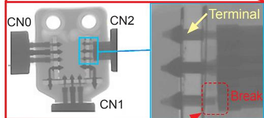
The internal circuit was broken.
