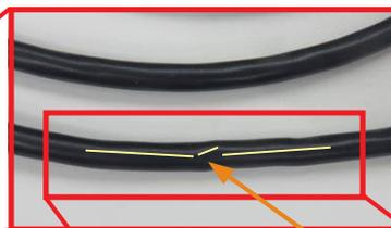
Cable sheath is deformed
