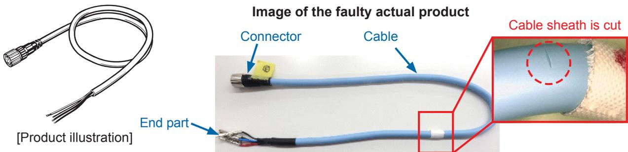
\* The target product uses a special cable cutter, and scratches such as those on faulty parts do not occur in the assembly process.
