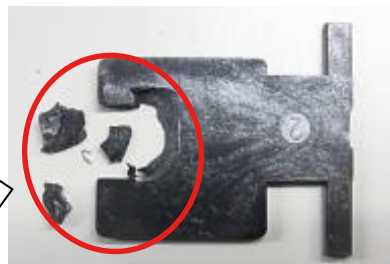
The lock plate is broken
