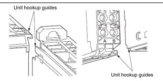
2 Slide the IO-Link Master Unit on the hookup guides.
