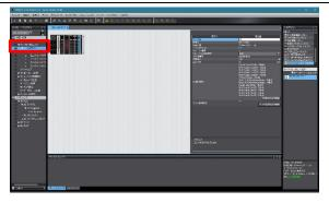
Right-click the IO-Link Master Unit displayed in the CPU/Expansion Racks area, and select IO-Link Master Simple Settings.
