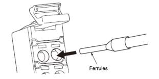
After making the connection, make sure that the ferrule is securely connected to the terminal block.
