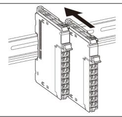
Press the IO-Link Master Unit with a certain amount of force against the DIN Track until you hear the DIN Track mounting hook lock into place.
