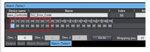
In this example, error code "4F" is displayed. The meaning of this error code is as follows.
