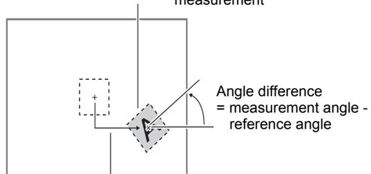
Position difference = measurement position - reference position
