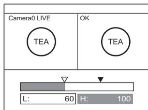
Select the target for input of the numerical values using the ← L key/→ R key, and press the SET key.
