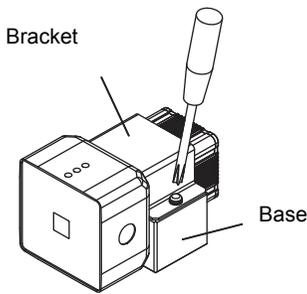
**1** Install the mounting fixture with the protrusion on its base (black) aligned with the groove on the camera body.
