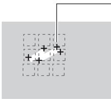
The extent of the defects is calculated in subdivided regions, and regions at or exceeding the defect threshold are output as the number of defects.
