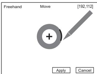
**4** If the profile is partially clipped, trace by [Free], [Box], [Ellipse] or [Line].
