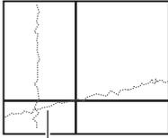
If the graph lines are inclined even though the measurement target illuminated as a uniform color on screen, you can judge that lighting is uneven.
