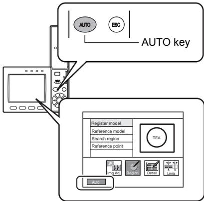
**1** Either press the **AUTO** key on the Controller or select **[AUTO]** on screen.
