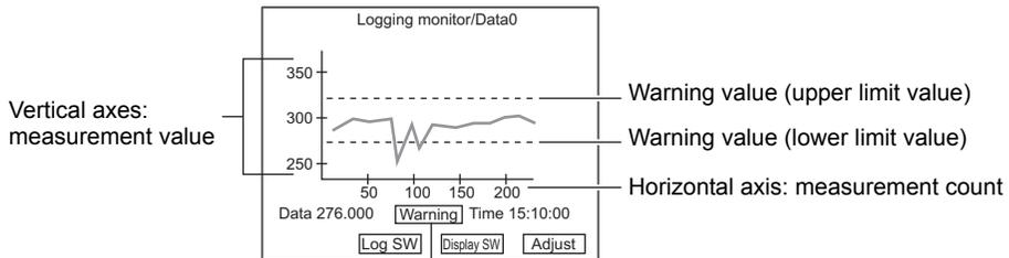
The warning is displayed when the measurement result falls below or exceeds the warning value.
