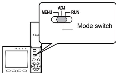
The ZFX-C has the following three modes. Switch to the desired mode before you start operation. To switch the operation mode, use the mode switch.
