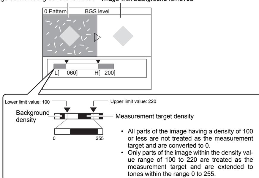
► MENU mode - [Setup] - [Item] - [Img Adj] - [Select camera] - [BGS level]
