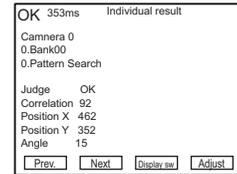
The 1/4 display is available only for the individual results display and position correction display.
