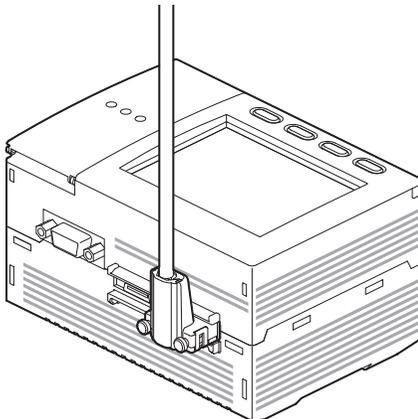
On the Controller side, the cable bends towards the rear.
