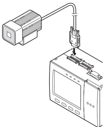
**1** Insert the camera's connector into the Controller's Camera connector.
