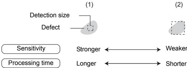
When a larger detection size is set, the difference with elements that are not defects decreases as the density of elements other than defects also is included in the calculation at (2). In other words, the more background that is included in the detection area, the weaker the detection sensitivity becomes.
