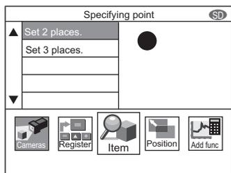
**1** Place the measurement target at the 1st point, and select either [Set 2 places.] or [Set 3 places.].
