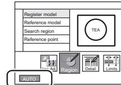
The optimum measurement conditions are automatically set just by selecting [AUTO]. Measurement conditions can also be checked and changed.
