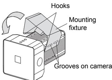
**1** Align the two hooks on one side of the mounting fixture with the two grooves on the camera body.
