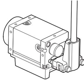
On the Controller side, the cable bends towards the front.
