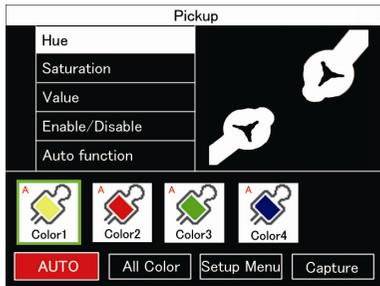
If the appropriate image is not obtained by automatic color pick up, fine-adjust three parameters hue, saturation and brightness. The image can be adjusted while comparing the picked up color image and original image.
