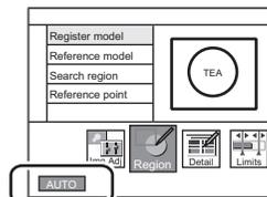
The optimum measurement conditions are automatically set just by selecting [AUTO]. Measurement conditions can also be checked and changed.
