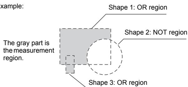
The shapes that can be selected differ according to the measurement item. Only selectable shapes are displayed.
