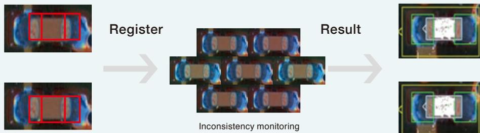
In order to cope with component inconsistencies, parameters can be automatically calculated - simply by registering required components.
