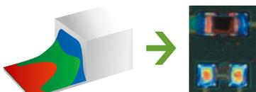
The Color Highlight technology provides a way of obtaining accurate information on solder joint angles in the form of image data.
