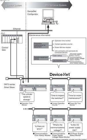
\*You cannot use the contact operation counter and the power ON time monitor at the same time.
