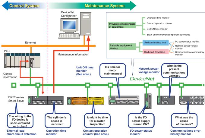
Note: The contact operation counter function and the unit ON time monitor function cannot be used simultaneously.
