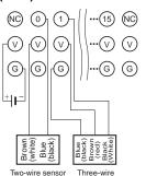
sensor with PNP output (e.g., photoelectric sensor or proximity sensor)
