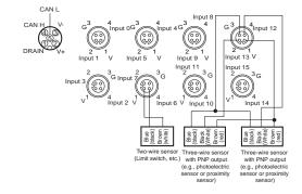
**Environment-resistive Terminals with Transistors (Standard Type)**
