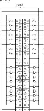
**Screw-less Clamp Terminals with Transistors**
