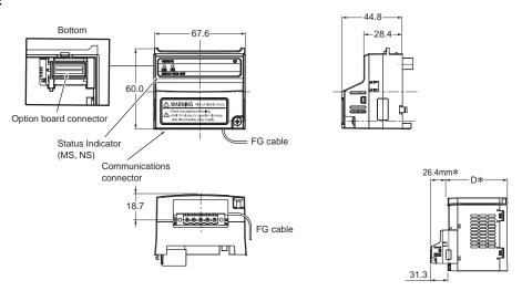
After the DeviceNet Communication Unit is installed, dimension D of the inverter increases by 26.4 mm (Dimension D of the inverter varies depending on the capacity. Refer to the MX2-series USER'S MANUAL (Cat.No.I585)) High-function General-purpose Inverters RX-Series V1 type DeviceNet Communication Unit
