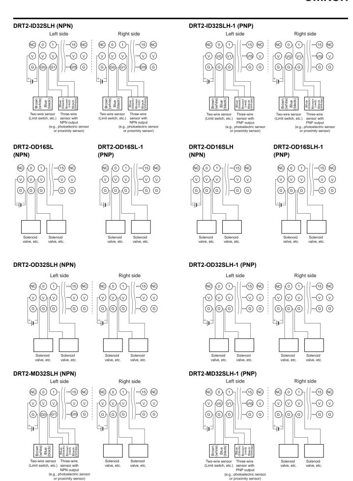
**Environment-resistive Terminals with Transistors (High-function Type)**
