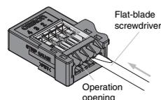
2. Insert the wire all the way to the back of the wire insertion opening. Confirm that the wire insulation has entered the wire insertion opening and that the end of the core has passed through the contact section.
