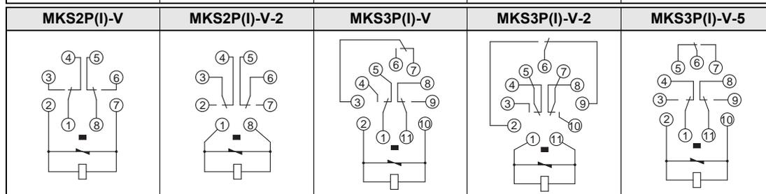
**Models with LED indicator and Varistor (AC Coil)**
