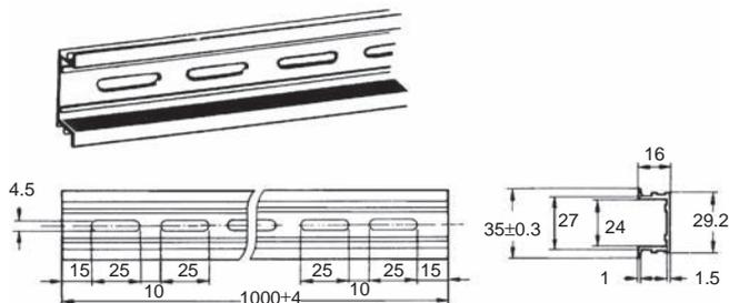
\* A total of twelve 25 × 4.5 elliptical holes is provided with six holes cut from each track end at a pitch of 10 mm.
