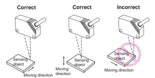
Install the Sensor as shown in the following illustration if each sensing object greatly differs in color or material.
