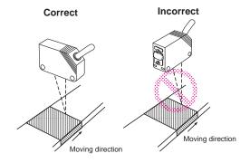
The stability indicator may turn off in reaction to reflection from background objects. In such cases, incline the Sensor by 10° as shown in the illustration for more stable detection.
