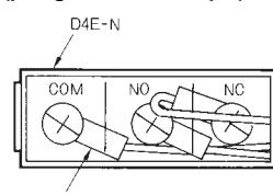
For the plunger and lever actuator models, the NC and NO terminal indicators are reversed.
