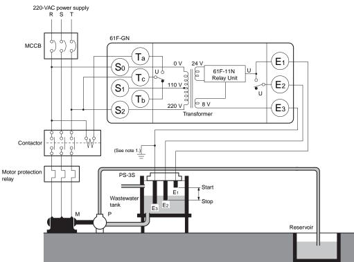
Note: 1. Be sure to ground the common Electrode E<sub>3</sub> (the longest Electrode).
