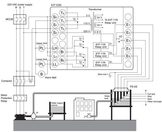
**Note: 1.** Be sure to ground the common Electrode  $E_5$  (the longest Electrode).
