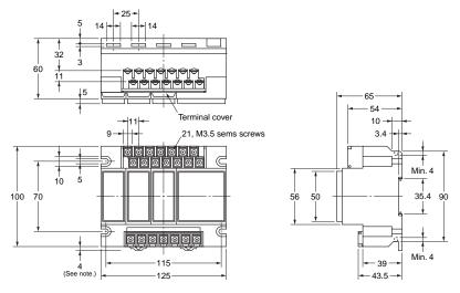
Note: Dimensions are with the DIN rail mounting (sliding) bracket attached.
