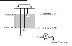
The pump starts (U indicator ON) when the water level reaches  $E_1$  and stops (U indicator OFF) when the water level drops below  $E_2$ .
