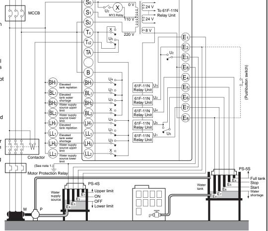
Note: 1. Be sure to ground the common Electrode E8 (the longest Electrode).
