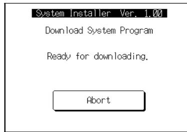
When the PT is in this status, transfer the system program from the computer's system installer.
