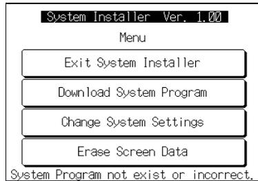
The system installer mode's menu will be displayed. When the system program is missing or corrupted, the message *System program not exist or incorrect* will be displayed.
