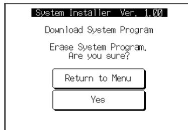
Press *Yes*. The system program will be erased. A message will be displayed while the system program is being erased.
