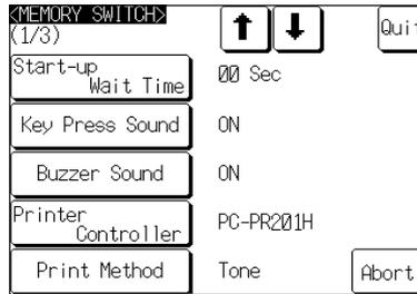
Press the **↓** touch switch (next screen) or **↑** touch switch (previous screen) to display the third memory switch setting screen.
