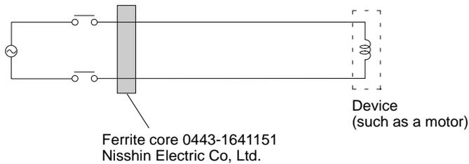
Because noise currents flow through metallic equipment (such as casings), the communications cables should be placed as far away from metallic equipment as possible.
