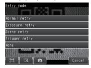
If you selected [Normal retry] or [Exposure retry], touch [Inspect] - [Retry details] and set the parameters.
