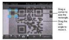
Check the area, press the [OK] Button, and then press the [TEACH] Button. The characteristic part and reference position for position compensation will be registered.
