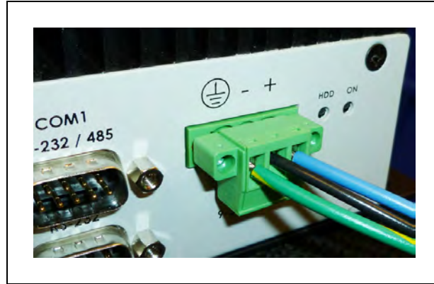
Figure 3-3. DC Connector with Wires
