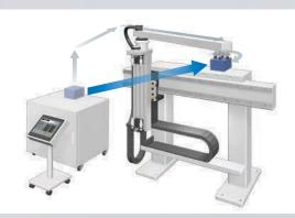
4-axis positioning function with linear interpolation
